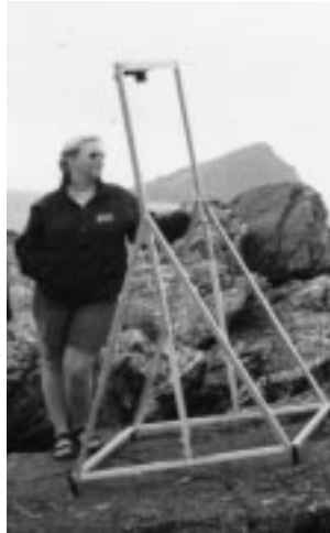
Figure 2 Quadrat in situ at Wembury VMCA during a survey. The lens used here was a 35mm, hence the height of the cross-bar camera supports.
