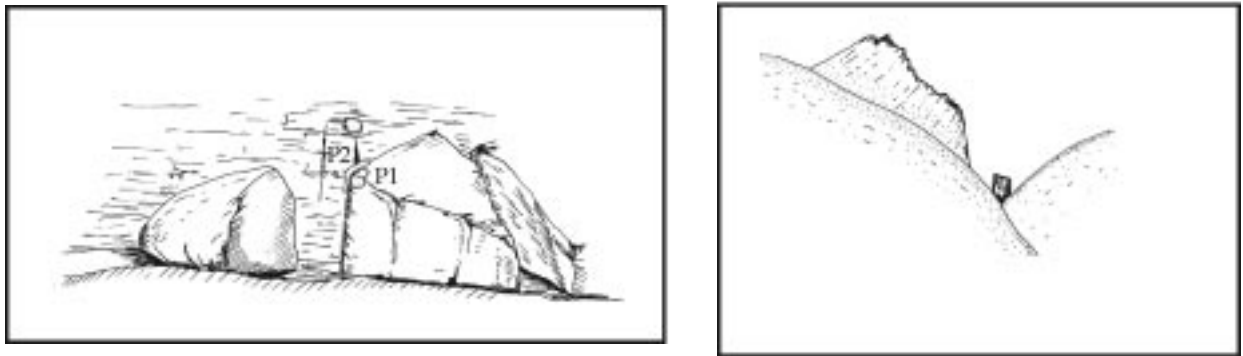
Figure 1 Drawings of marks and transit features. On the left, when the paint marks (P1 & P2) on a foreground boulder and background cliff face are correctly aligned will indicate the correct location in terms of position and distance offshore. On the right, the transit features are correctly aligned when the tooth-shaped rock appears in the 'V' of the hillside.
